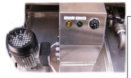
Loading of the oil into the fryer automatically (controlled by MAX and MIN levels) or manual.
