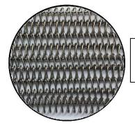
Fryer tape and counter-tape for immersion products made with stainless steel mesh type TN, as in the picture.
