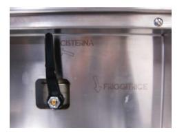
It is possible to decide whether to send the filtered oil to the fryer's tank or to the oil recovery tank (see image). If you drain it in the oil recovery tank, you can keep it at the set temperature (thanks to an adjustable thermostat) so as to keep it in a liquid state, ready to be used immediately.
